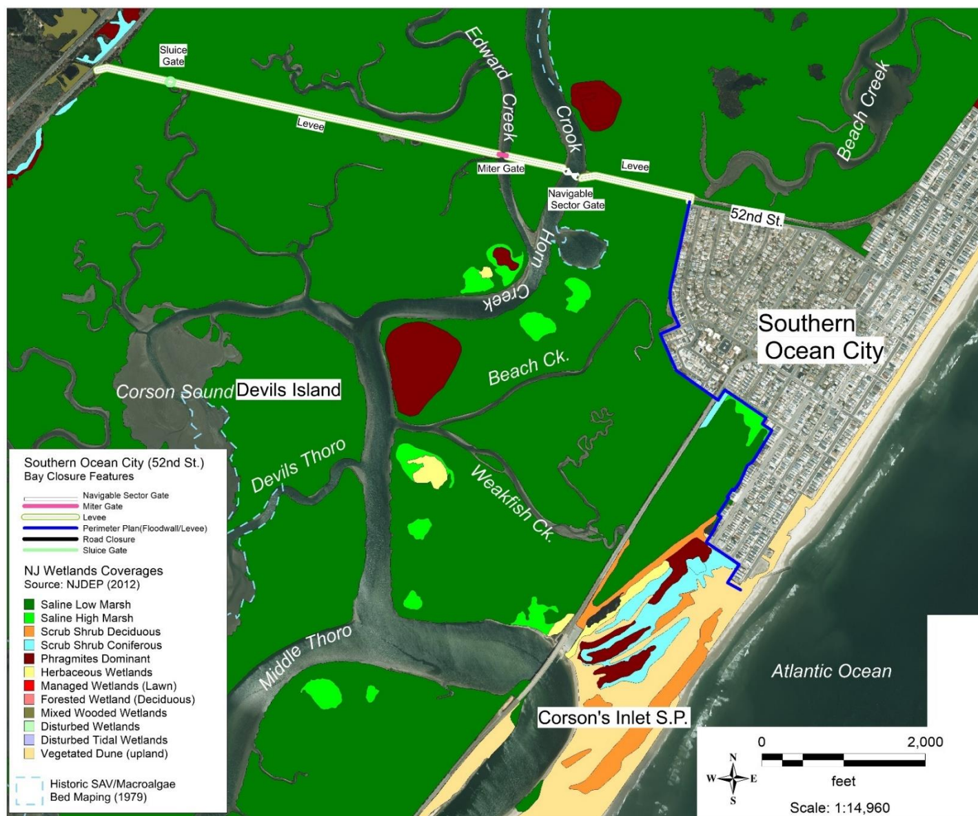
Figure 107: Alignment of the Southern Ocean City Cross-bay barrier (CBB) and Features with Wetland Habitats
