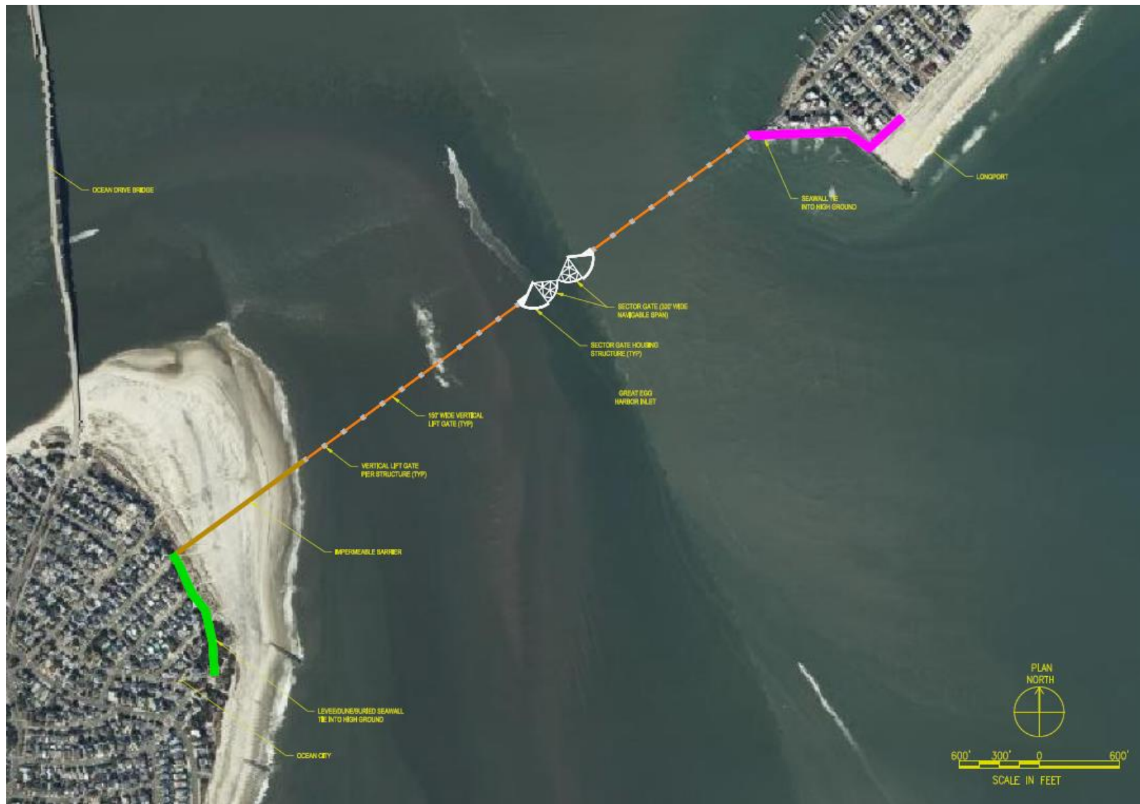
Figure 73: Great Egg Harbor Inlet storm surge barrier plan view
